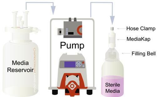
**Figure 4** Operation with peristaltic pump
