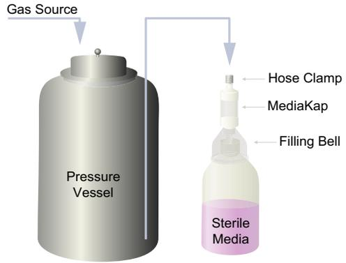
**Figure 3** Operation with pressure vessel
