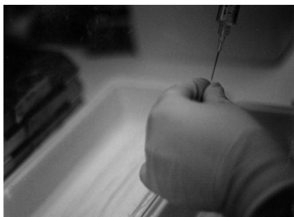
Figure 1: Filling of the equilibrated KrosFlo® Implant Membrane hollow fibers. A syringe, filled with the cell suspension, is attached to a hollow fiber by a needle, PTFE catheter or pipet tip. The fiber is flushed with the cell suspension. The fiber is sealed on each end with hot smooth-jawed needle holders and the individual samples are prepared by cutting at each heat seal. The prepared samples are transferred to culture dishes containing growth medium for incubation.
